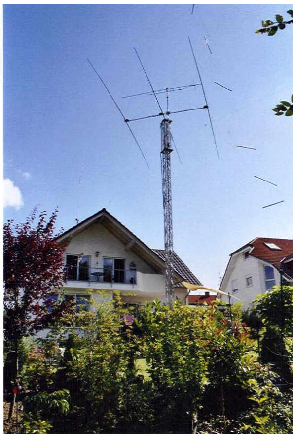
Fig. 7 – Vertical part of the „invisible antenna“ with the PVC insulators, including now also the 40m radiator.
