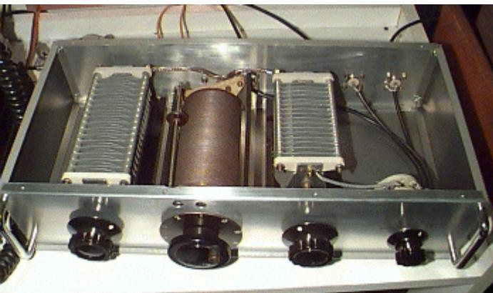
If you follow the basic guidelines given here, you should be able to build a useful ATU for your station at minimal cost. This picture shows my ATU with the top panel removed, a pair of 50 Ohm dummy load resistors were also removed to show the connector placement (right side behind switch block).
