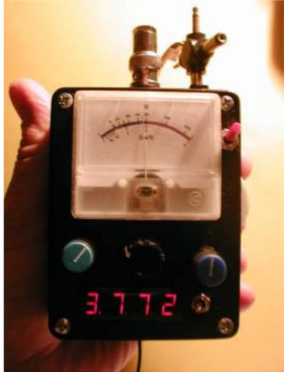
The completed “Mk1” antenna analyser
